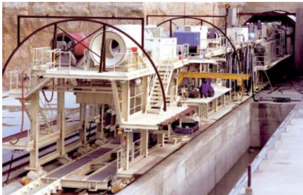
"La Adelantada" tunnel-boring machine.
