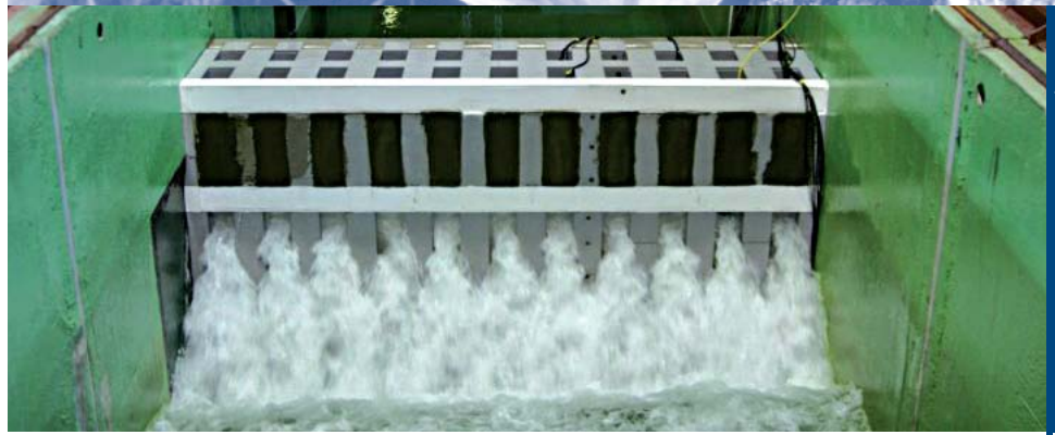
Low reflection caissons for wharves and seawalls
